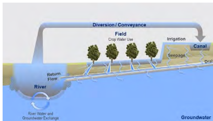
FIGURE 10: Schematic of Rio Grande and Groundwater System Interaction Prior to Development of Groundwater Pumping in Rincon and Mesilla basins
